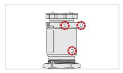
The Z-SPOT features three M4 mounting points spaced along its body, providing versatile options for securely attaching and mounting the product. For the 3rd M4 mounting point, a 1.8mm thick M4 washer is required to ensure proper installation and stability.
